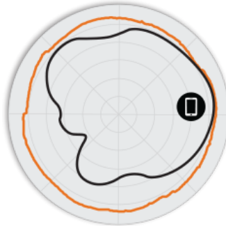
Figure 3. T610o 5GHz Azimuth Antenna Patterns
