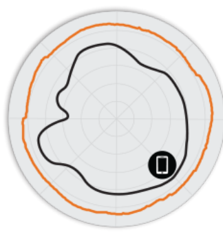
Figure 3. R850 5GHz Azimuth Antenna Patterns
