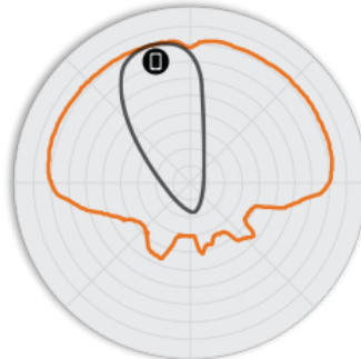
Figure 4. H320 2.4GHz Elevation Antenna Patterns
