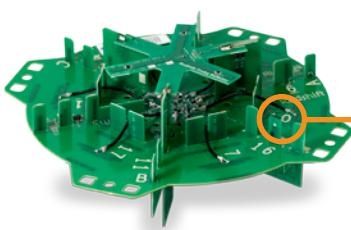
A patented smart antenna array in each Ruckus Smart Wi-Fi outdoor AP integrates horizontally and vertically polarized high-gain, directional antenna elements to provide over 4000 potential signal paths to any given end device while delivering up to 7dBi in signal gain and up to -15dB of interference avoidance for unprecedented range extension, signal reliability and higher data rates.
