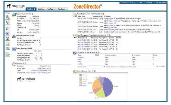
As part of a centrally controlled wireless LAN, the ZoneFlex 7321 is managed through an highly intuitive and simply to use graphical, point-and-click Web interface. The dashboard (below) gives administrators a single and comprehensive view of the state of the wireless LAN.
